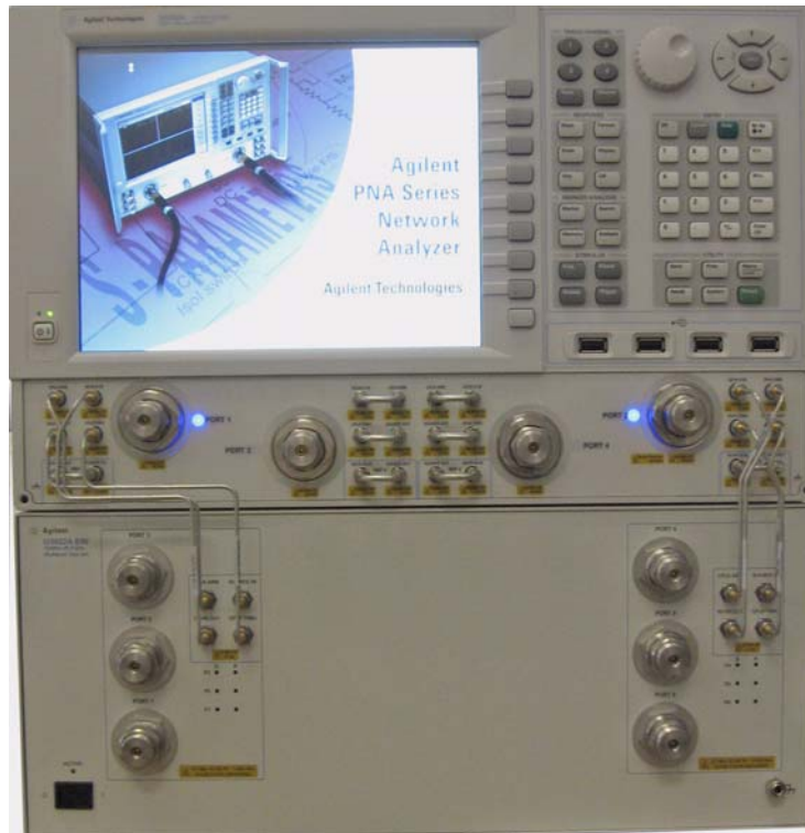
Figure 2 N5242A 4-Port PNA-X with U3022AE06
